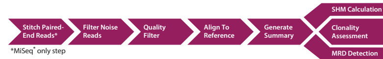
FIGURE 2. BIOINFORMATICS WORKFLOW LymphoTrack® bioinformatic analysis begins on MiSeq® with stitching of paired reads (PGM® analysis begins at the next step). The resulting sequence file is then filtered for noisy reads (non-specific or fragments that are too short), and reads that do not pass quality are removed. These reads are then aligned to the reference sequence database, and numerous statistics are calculated. SHM rate is calculated from the alignable portion of the V-gene. MRD detection requires the previous identification of a clonal read, and for the user to input the amount of DNA being assayed. MRD results are reported for exact matches, and very similar matches to the clone submitted by the user. A confidence value is assigned to these results that tell the user the reliability of result, which is based on how much DNA was assayed, as well as the read depth achieved for that sample. The confidence is based on theoretical samplings using a binomial distribution.
